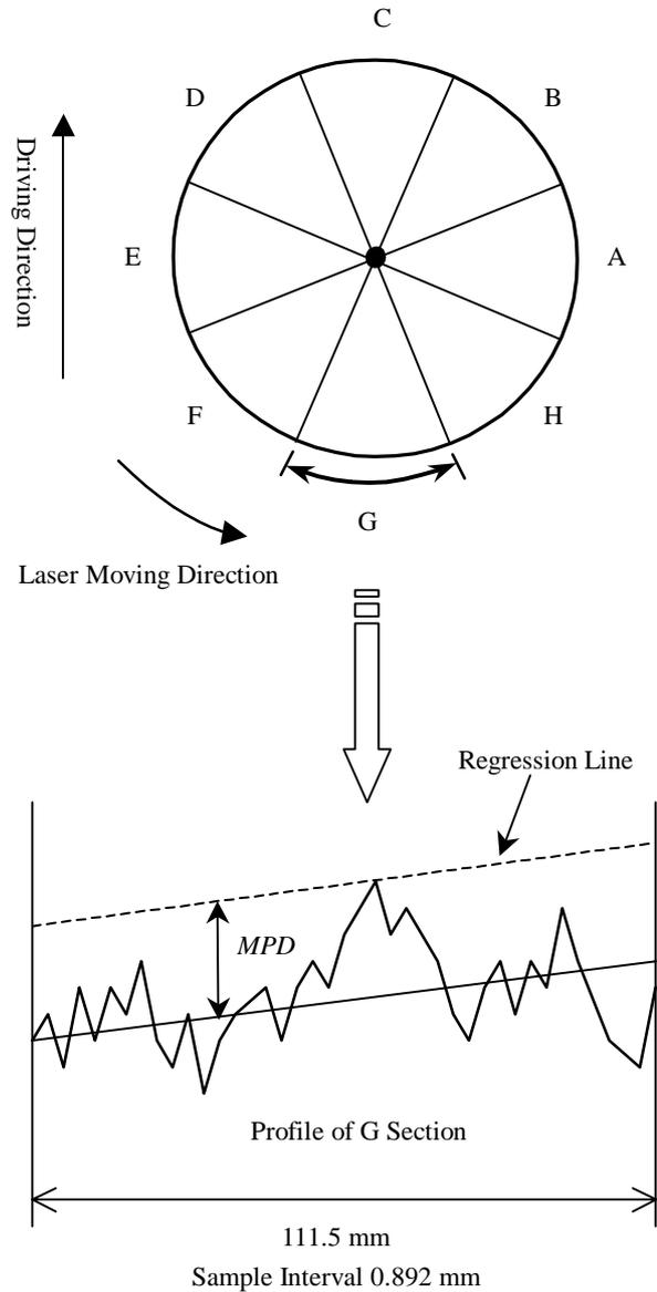
Figure 2. Calculation of MPD from CTM Measurements
